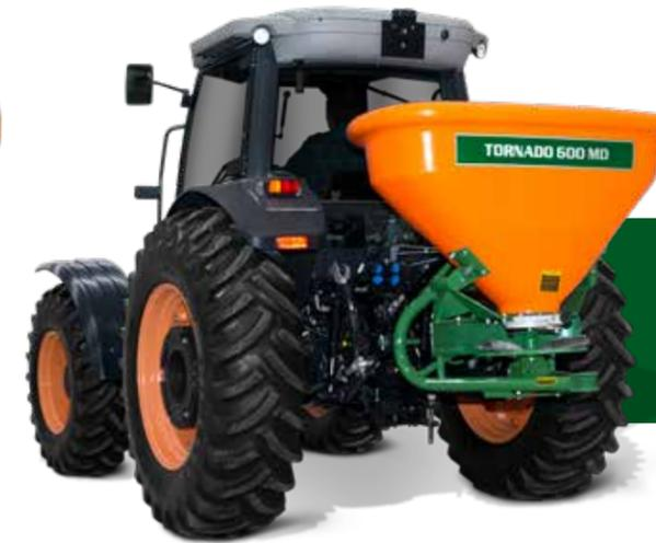
The gravity center of the load closer to the tractor allows to work without the need for front weights avoiding toppling
