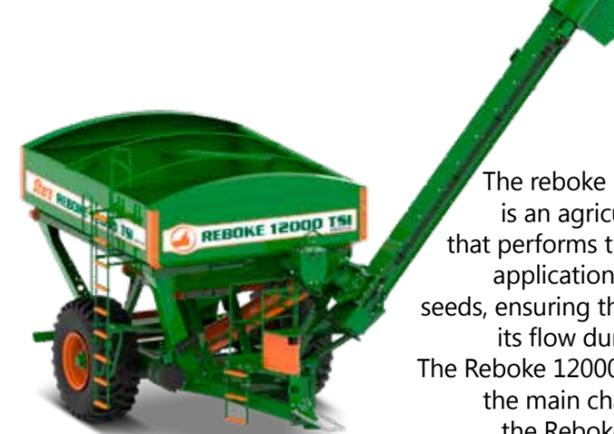
The reboke 12000 TSI Grafite is an agricultural chaser bin that performs the instantaneous application of graffiti on the seeds, ensuring that the seed have its flow during the planting. The Reboke 12000 TSI Grafite keep the main characteristics from the Reboke 12000 TSI.
