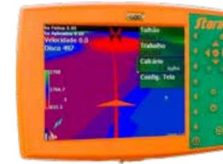
Twister 1500 APS can be equipped with the Topper 4500 controller that works with a free or paid signal, and can be used in fixed or variable rate applications. Dosing information is sent to the electric center that adjusts the application rate through sensors and electric motors.
