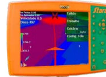
The Twister 5500 can be equipped with the variable rate system. The controller Topper 4500 works with free or paid signal and can be used in the variable or fixed rates. The dosages information are send to an electrical central that through sensors and electric gate, allows varying the application rate.
